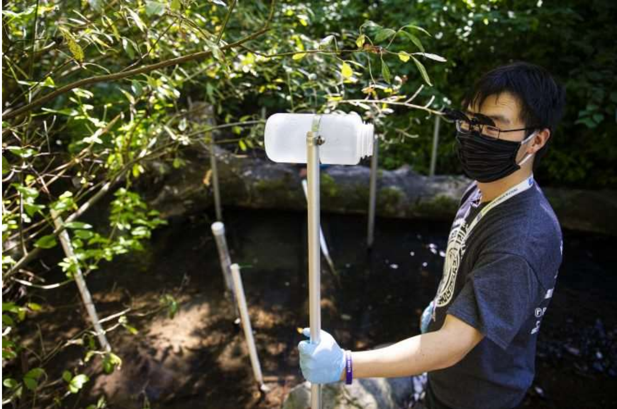
Caption: Zhenyu Tian is holding a sampling pole, which is used to collect creek water for future tests. Credit: Mark Stone/University of Washington
